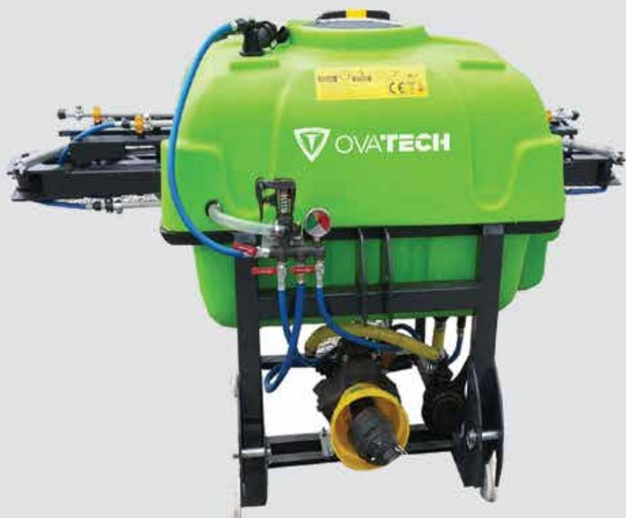
Tractor mounted sprayer by PTO via shaft developed to meet the different requirements of plant protection
